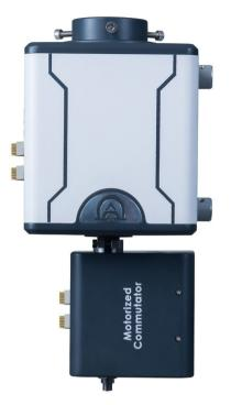
The Alpha Omega **Alpha Commutator** is a motorized slip ring commutator that facilitates smooth tethering to research animals. It supports both neural recording and stimulation. The commutator actively tracks the rotation of the headstage cable and compensates, eliminating turn-induced torques on the research subject.
