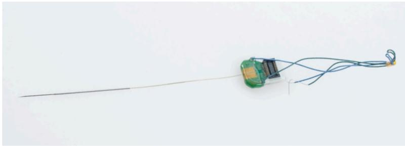
The **Chronic Vector Array™** is a design enabling access to deep brain structures (> 10 mm deep) for chronic applications.
