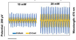
Time: 10 ms Distance: 250 µm from electrode
