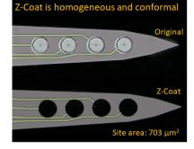
Z-Coat reduced impedance and noise improves the recording capability of microelectrode arrays, giving the advantage of smaller amplitude signal detection. Z-Coat improves the signal-to-noise ratio which allows researchers to peer further into the tissue to detect low amplitude signals that are typically buried in the noise when using conventional electrode materials.
